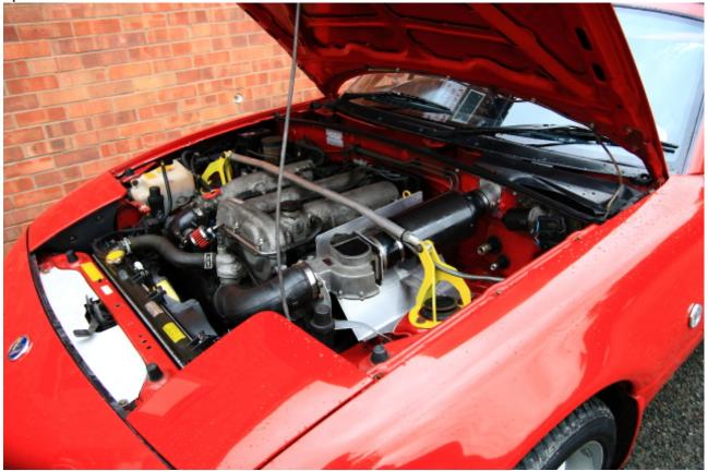
I also did a few under bonnet modifications, fitted a strut brace and routed the induction to the scuttle panel to harvest cooler air.
